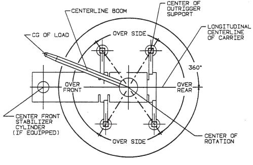
BOLD LINES DETERMINE THE LIMITING POSITION OF ANY LOAD FOR OPERATION WITHIN WORKING AREAS INDICATED
